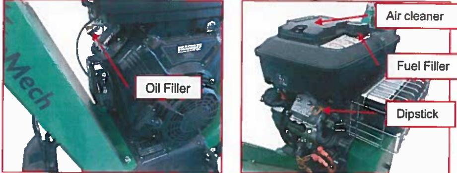
Fig 6.2b Engine Oil, Fuel, Air cleaner – CS 80 Loncin– view each side
