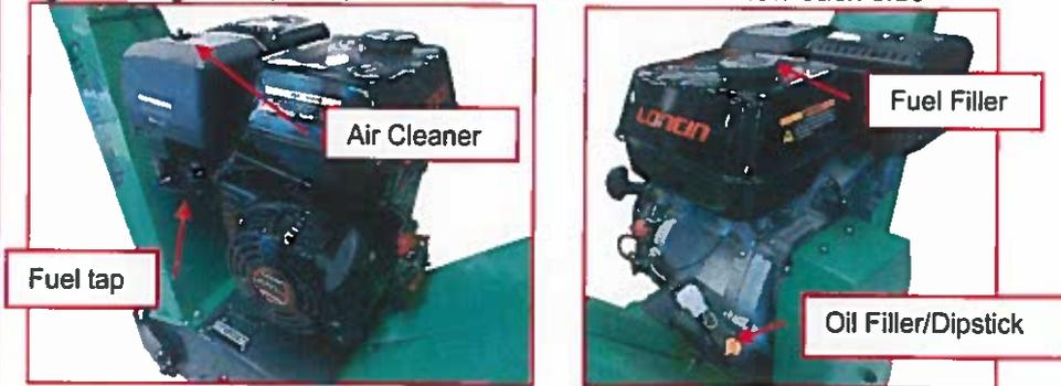
**6.3 Fuel Level** Refer to Fig 6.2a or Fig 6.2b depending on engine type. Check daily before work and fill as required (fig 6.2).
