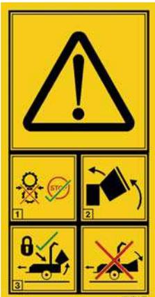
**Do NOT fold infeed chute unless control bar is in STOP position**
