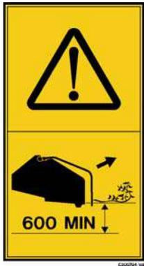
**Do NOT operate with infeed chute at less than 600mm from ground (bottom bar machine).**
