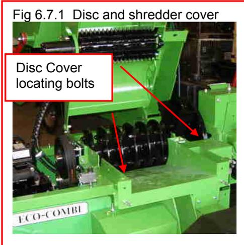
Fig 6.7.2 Discs and disc blades
