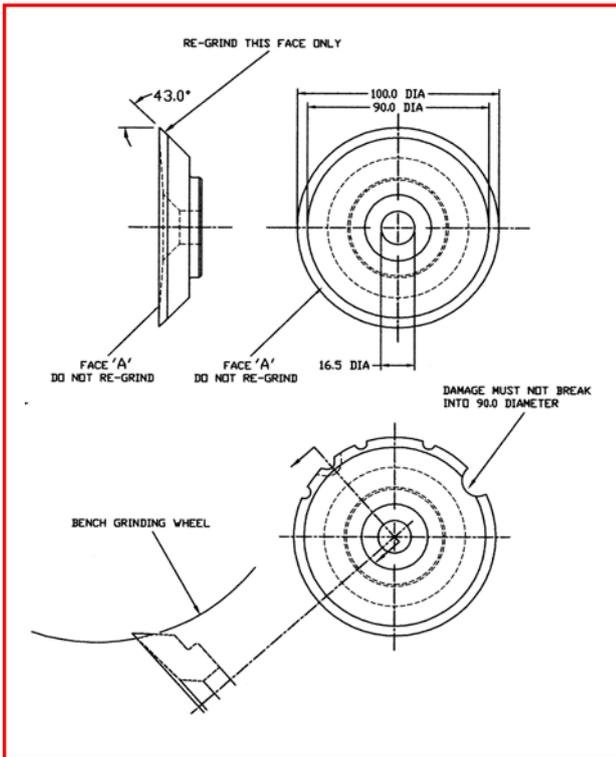
6.24.1 Examine set of chipper discs for damage. If front face 'A' is worn the disc must be scrapped. If chips have broken off the cutting edge they can be re-dressed provided that they do not go inside the 90mm diameter.
