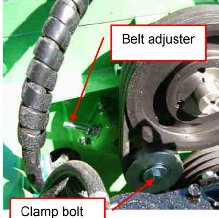
Fig 6.9b Drive belt tension
