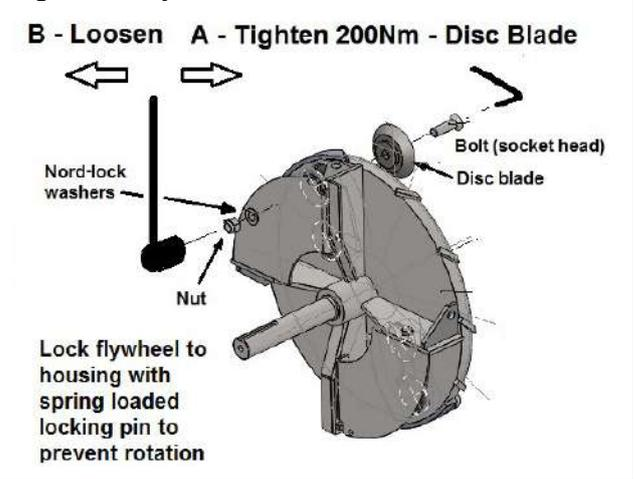
Fig 6.7.3 Blade fastening assembly
