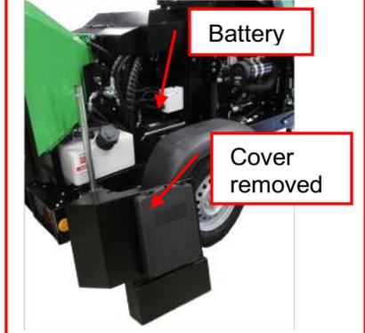
**⚠ CAUTION! Gases are explosive. Electrolyte is corrosive. Avoid sparks and spillage.**
