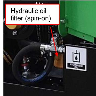
Hydraulic oil filter (spin-on)
