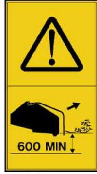
Do NOT operate with infeed chute at less than 600mm from ground (bottom stop bar).
