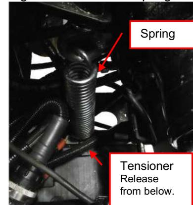
Fig 5.4.2 Feed roller lift
