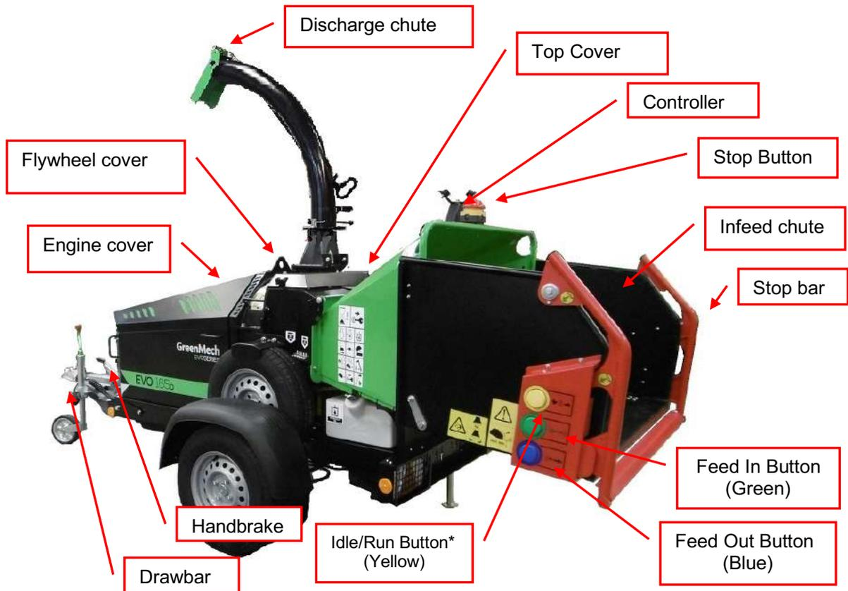
Fig 2.1 EVO165DT Track model Main Features
