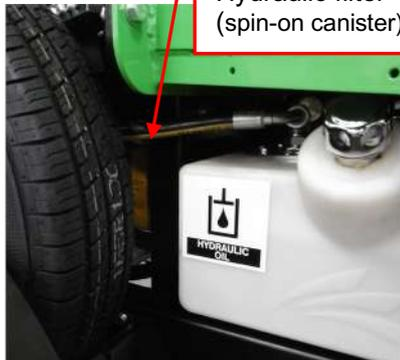
Hydraulic filter (spin-on canister)
