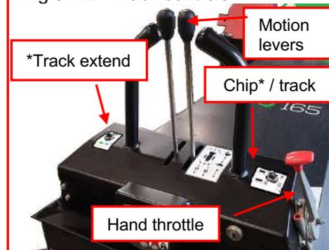
**Note:** Drive with track motors at rear when possible.
