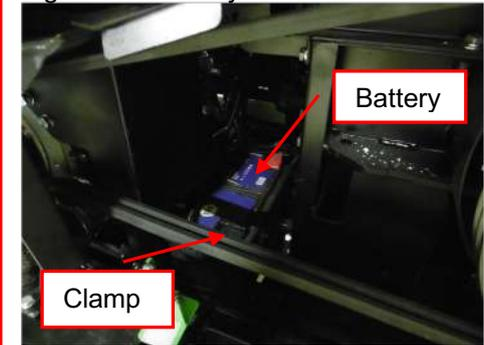
**CAUTION!** Gases are explosive. Electrolyte is corrosive. Avoid sparks and spillage.
