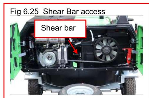
Fig 6.25 Shear Bar access
