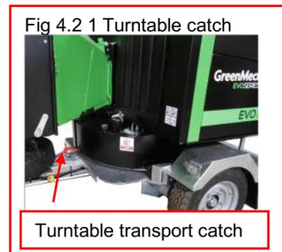
**CAUTION!** Before travelling, ensure that turntable is rotated back into transport position, locked and secured with transport catch.
