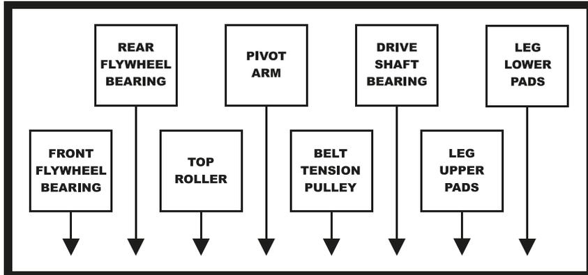
Left to Right on remote manifold – 8 grease points 6.1.2 >> 6.1.9.
