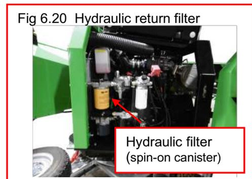
Fig 6.20 Hydraulic return filter
