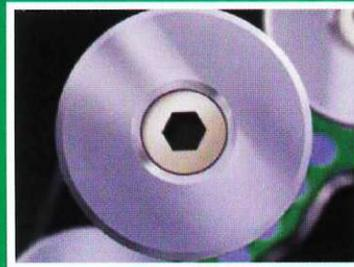
By loosening the retaining bolt the Disc-Blades can be rotated in either direction. If damage occurs to the blade through insertion of contaminants i.e. stones, nails etc the damaged section can simply be positioned away from the cutting area.
