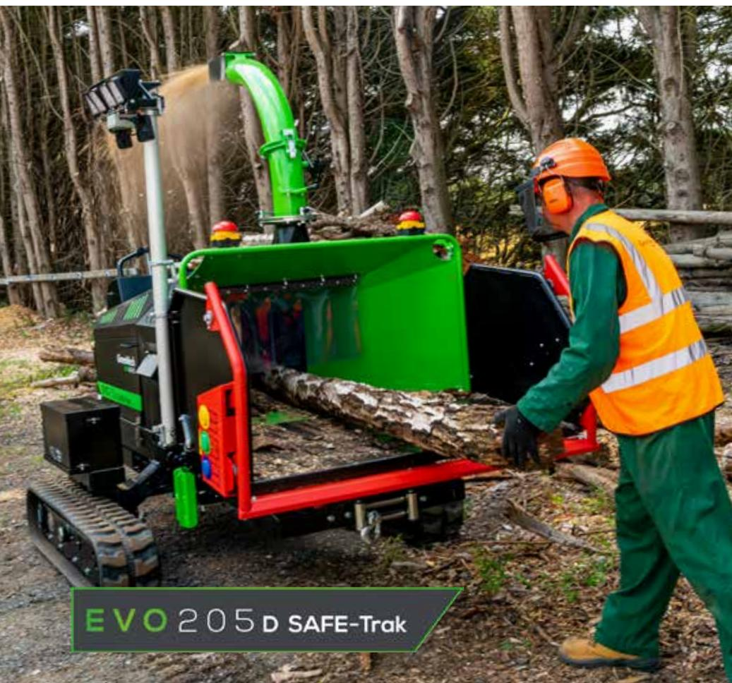
The EVO 205D SAFE-Trak is designed with GreenMech's patented and award-winning track extension system, allowing ground clearance of up to 400mm enabling access across the most difficult terrain. This pioneering feature makes it popular for de-veg contractors working on power line and railway track maintenance.
