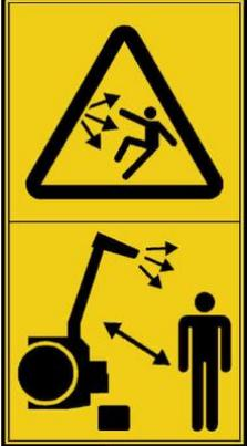
**Action: Keepaway from fast discharge chute**
