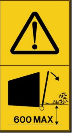
**Do NOT operate with infeed chute at more than 600mm from ground (top bar machine).**
