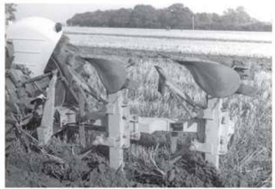
**Left: A 1966/67 Track Marshall 70C holding aloft a Turner four-furrow, fully-mounted reversible plough. The three-point linkage was designed by Roger Dowdeswell and made and marketed under license by Turner Engineering.**
