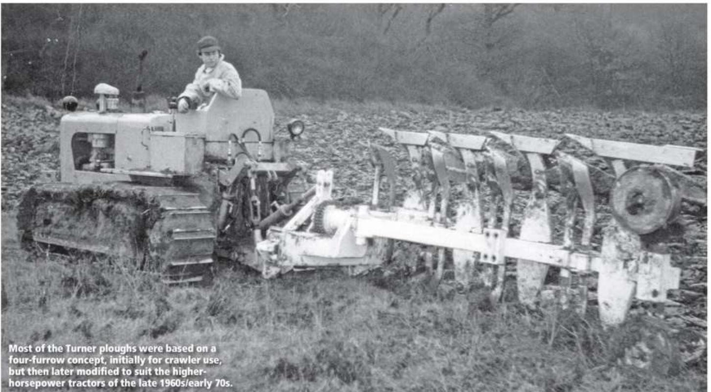
Most of the Turner ploughs were based on a four-furrow concept, initially for crawler use, but then later modified to suit the higher-horsepower tractors of the late 1960s/early 70s.
