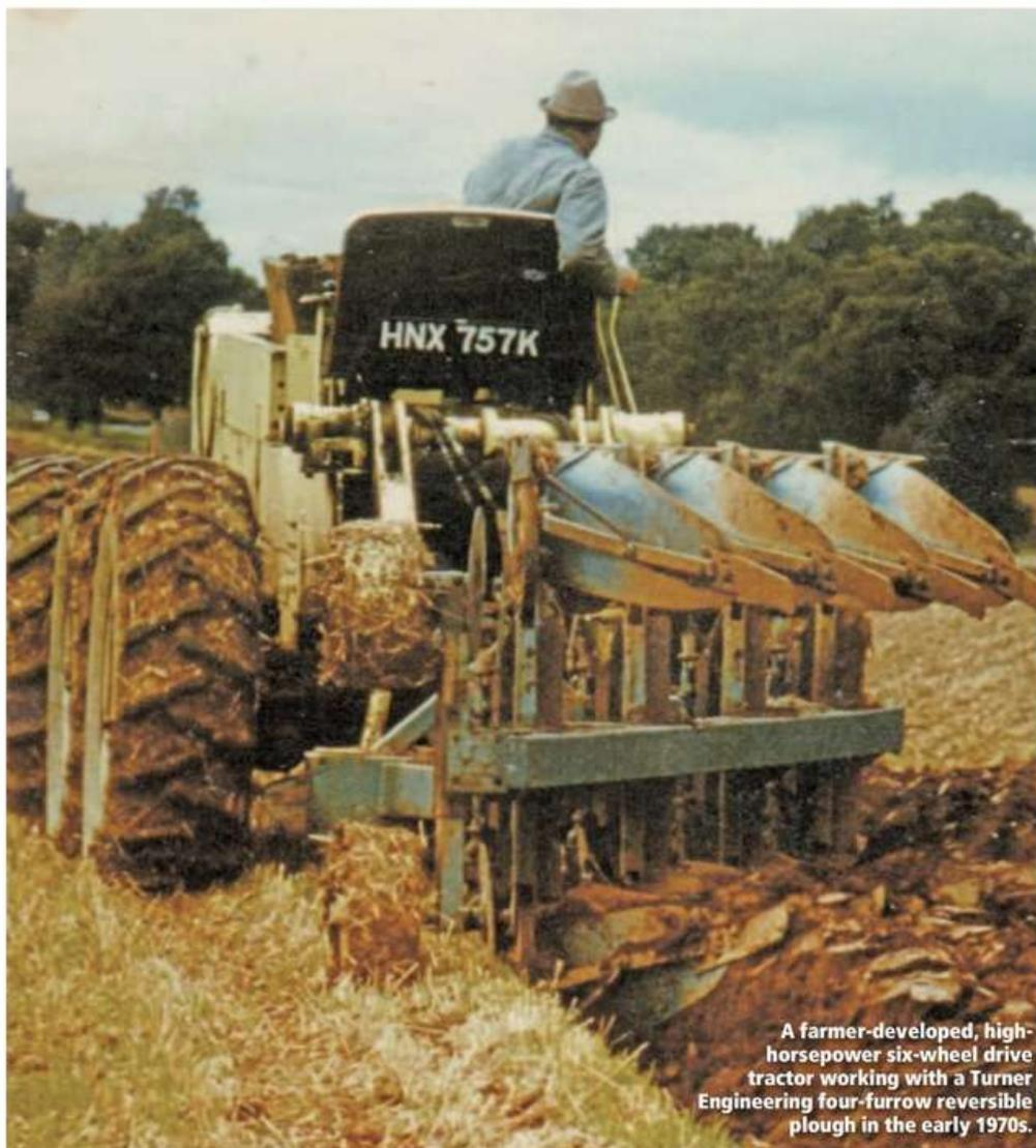
A farmer-developed, high-horsepower six-wheel drive tractor working with a Turner Engineering four-furrow reversible plough in the early 1970s.
