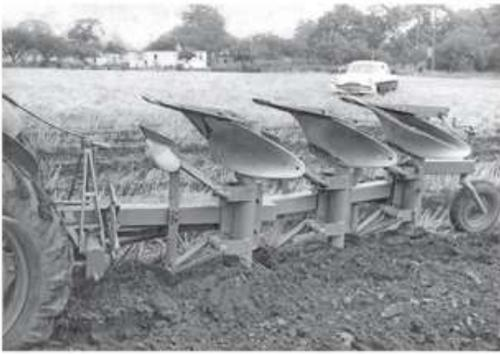
**Above:** Bomford Bros introduced a three-furrow, semi-mounted reversible plough in 1963. It went on to make 95 three-furrow ploughs between 1963 and 1967, the latter year being when plough production ceased, and 24 four-furrow variants.
