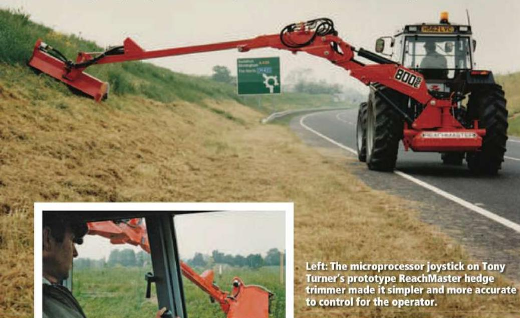
Left: The microprocessor joystick on Tony Turner's prototype ReachMaster hedge trimmer made it simpler and more accurate to control for the operator.
