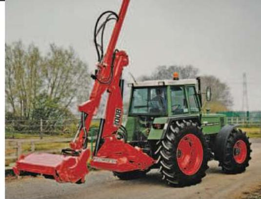
Above: The flail head and arm of the ReachMaster tucked in behind the tractor during transport. Before commercial production commenced, the entire project was purchased by a Danish company in the late 1980s.
