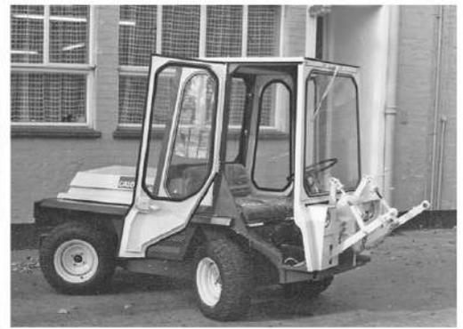
**Above:** The optional front or rear three-point linkage for the Ranger came from the Leyland 154. The Ranger was also available with front and/or rear PTO.
