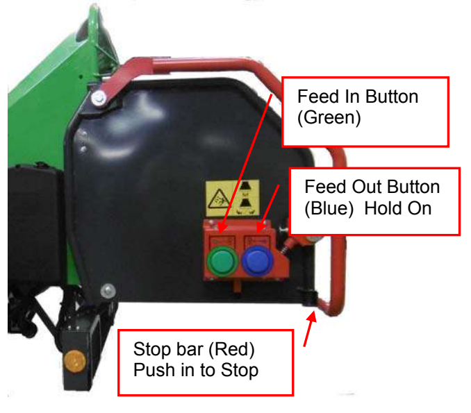
Fig 3.4.1 Stop Bar and Feed control Buttons
