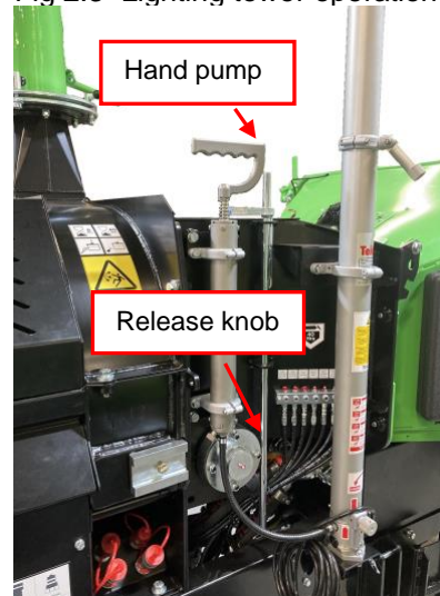
Fig 2.3 Lighting tower operation
